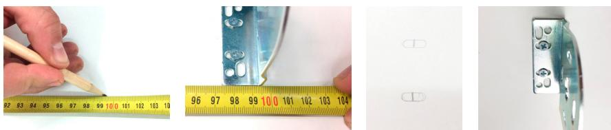
**NOTE:** It is important to attach the supports when they are well centred, as this way, if there is any deviation in the measurements, the supports can be moved to adjust the position.
