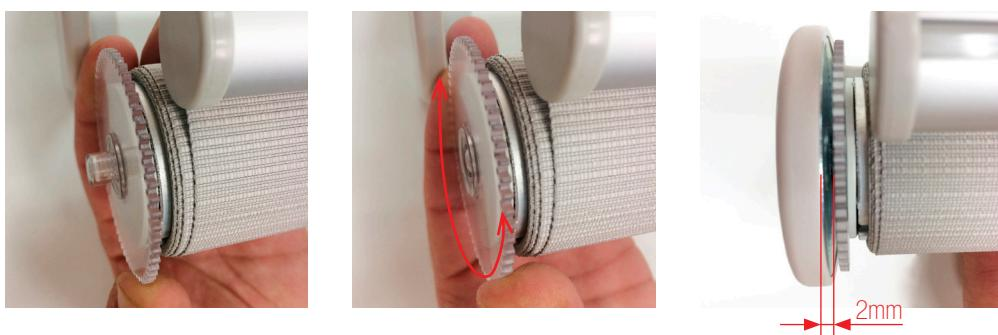
**NOTE:** The suitable separation between the support and the "one touch" must be 2 mm. Otherwise, remove the blind and move the supports as necessary to achieve this distance.
